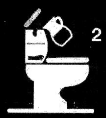
REMOVE THE TANK LID AND FILL IT WITH WATER UNTIL IT REACHES THE OVERFLOW LINE
